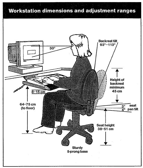
This drawing shows the recommended dimensions and adjustment ranges for the chair, monitor, keyboard, and work surfaces. The operator in this drawing is using good posture.
